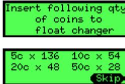
Insert the requested coins into the changer through the discriminator, the count of how many coins are required will decrease as coins are inserted. When sufficient quantity of a coin have been inserted it will stop prompting for that coin and reject any more that are inserted.
