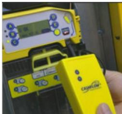
Before doing any further steps update the software, coinset and product options using a CPM loaded with the appropriate applications (CPM files).
