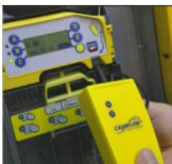
Delete any existing acoustic calibration data in the changer by using a CPM loaded with a special application to perform this function. Plug the CPM into the changer, wait for the download to complete and the changer to restart.
