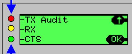
**Green** LED is ON when the printer indicates BUSY (CTS) i.e. it is unable to print
