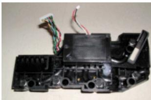
Pull the acoustic module forwards and remove it, dispose of appropriately.
