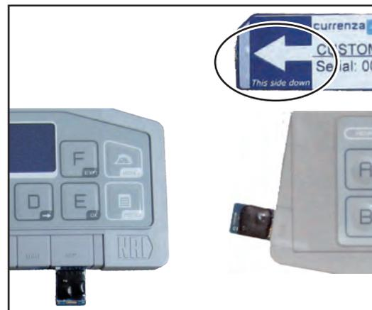
**Fig. 2:** Inserting SIM card
